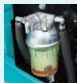
Pre fuel filter with built-in water separator
